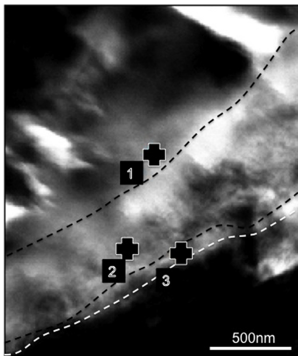
Fig. 4 – The image of GIC/dentin interface with polyalkenoic acid conditioning after 1 week storage as captured by FE-TEM. Plot 1 indicated the GIC area, Plot 2 indicated the IL area and Plot 3 indicated the ML area.
