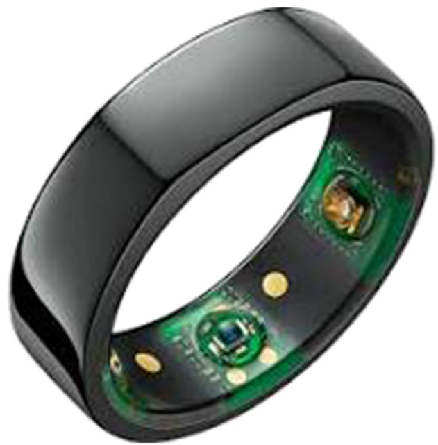
Fig. 1 The Oura sleep tracking ring. The sensors — infrared photoplethysmography (PPG) for heart rate, negative temperature coefficient (NTC) for temperature, and 3D accelerometer for movement — are placed on the inner surface of the ring
